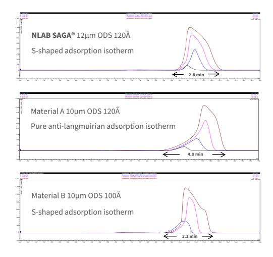
Loading comparisons from analytical up to preparative scale of an 8 A.A. cyclic peptide shows the narrowest band broadening for NLAB Saga®, indicating NLAB Saga® having the highest loading capacity.
