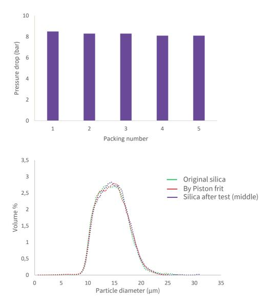
A DAC column with an internal diameter of 5 cm was used. 5 packings/unpackings to 100 bars were made with the same silica slurry. The mechanical stability test was performed on unbonded silica. Packing and unpacking of silica in a DAC column at 100 bar is a generally accepted test of mechanical strength of silica. Minimum back pressure drop over packing cycles and unchanged particle size distribution indicates a high mechanical stability of NLAB Saga.
